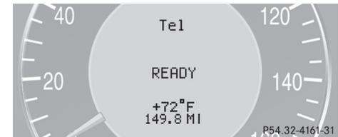
This standby message indicates that your telephone is ready for use and you can operate it using the control system.
