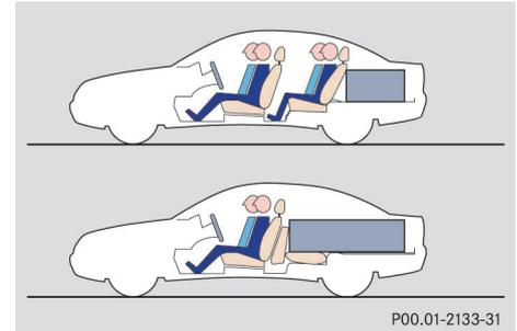
The total load weight including vehicle occupants and luggage/cargo should not exceed the load limit indicated on the corresponding placard located on the driver's door B-pillar (▷ page 316).
